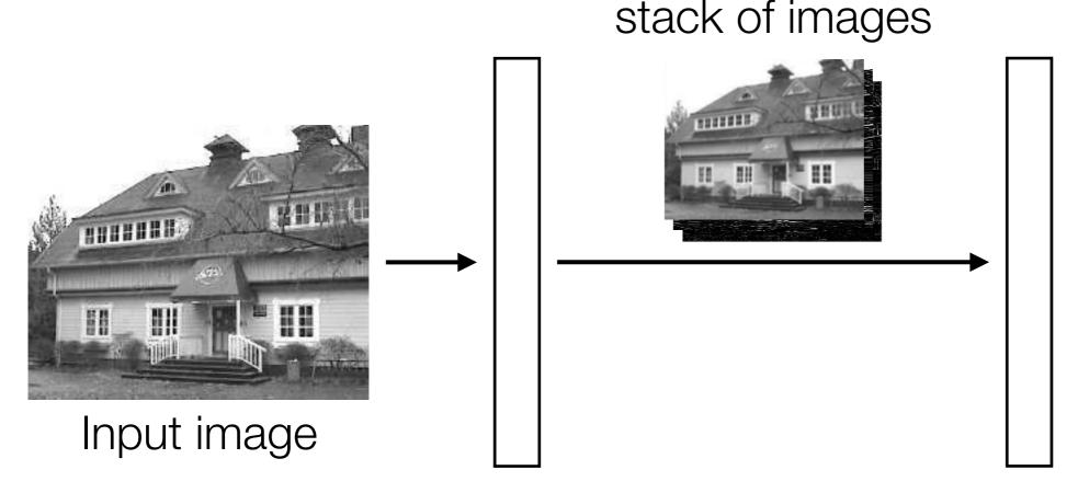
conv2d layer with ReLu activation and *k* kernels max pooling (applied to each image in stack)
